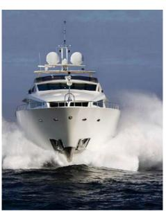
Available in an array of dish sizes ranging from 48 cm to 95 cm, the NT-Series line of satellite TV antenna systems is optimized for Ku-band TV reception at sea.
